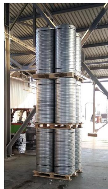
Рис.2 Metal drums in a "column" stack
